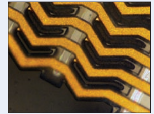
2006 Parylene-insulated gold lead structures are realized to enable folding microsystems for the first time.
