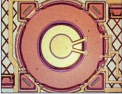
2000 A vacuum-sealed pressure sensor used to allow closed-loop control of an 8b integrated flow controller.
